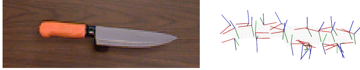
Figure 5.2: Left: knife; Right: Grasp candidates all across the knife. Cognitive affordances can serve as a normative constraint when selecting one of these many possible grasp possibilities.
